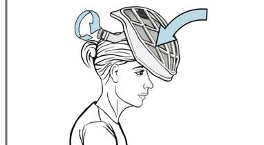
**Put helmet on head and size to fit by turning ratchet knob to adjust the headband.**
