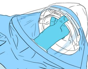
**Slide the helmet into the hood until it snaps in the center hole. Snap helmet into the hood on the left and right side snaps of the face shield.**
