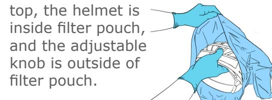
**Take off the helmet and place it inside the PAPR hood. Ensure the white HEPA filter is on top, the helmet is inside filter pouch, and the adjustable knob is outside of filter pouch.**
