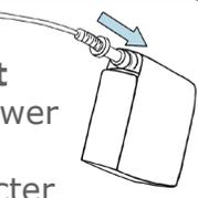
**Insert** the power cord connector into the battery.
