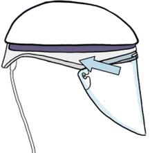
**Attach** the left and right side lens cuff mounting holes over the left and right side attachment posts of the helmet.
