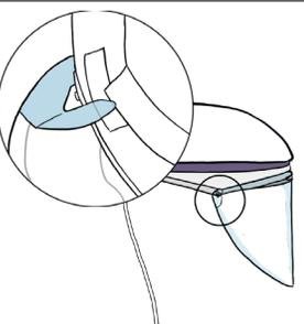
**Lift** the cuff flappers to rest against the foam pads at the ends of the comfort strip.
