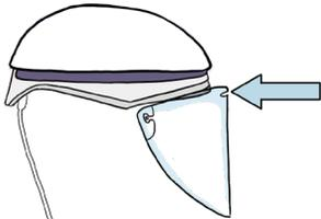
**Secure** the lens cuff by **aligning** the center hole over the center attachment post on the helmet.
