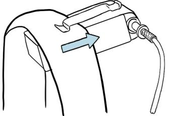
**Secure** the battery to the belt using the battery clip.
