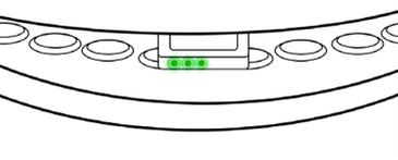
**Check** the LED lights to ensure the battery is fully charged.
