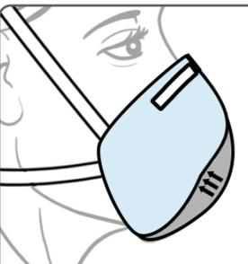
**Ensure** that the face piece collapses slightly under negative pressure that is created with this procedure.
