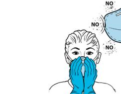
If the air leaks out between your face and the respirator, the respirator does not fit your face properly.
