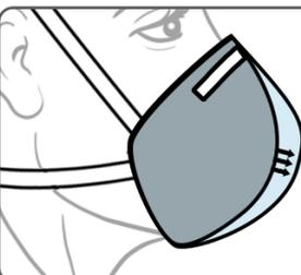
**Ensure** that the face piece is slightly pressurized before pressure causes outward leakage.
