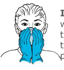
**Inhale** sharply while blocking the paths for air to enter the face piece.
